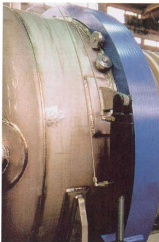
Electric hydraulic opening of vessel
