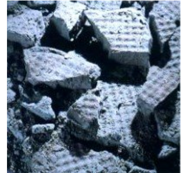
Typical sludge cake contains up to 75% water
