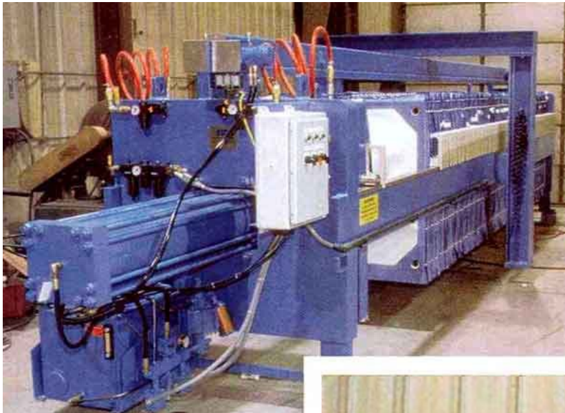
Durco EP Filter Press using hydraulically operated chain-drive filter plate shifter with double pawls
