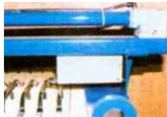
6 As the Shifter Assembly contacts the end stop, the pawl lifts up into the assembly in an unlocked position.
