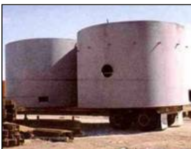
API 650 Storage Tank
